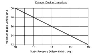
This damper's design at a length of 60" has a maximum allowable blade deflection of L / 360 for the static pressure indicated on the chart. At reduced blade lengths, higher static pressure limits can be attained without sacrificing damper operating performance characteristics.
